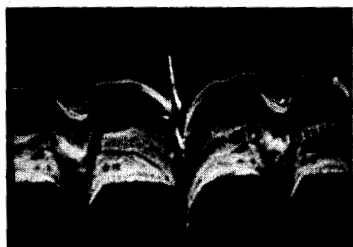
Fig. 3-13. Hum in the video-IF signal.
