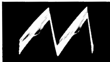
Fig. 5-5. Sawtooth waveform from horizontal-oscillator circuit, when coupling capacitor is leaky.
