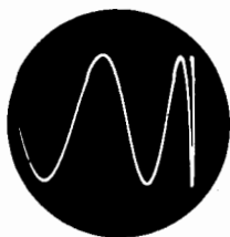
Fig. 1-27. Severe horizontal nonlinearity.
