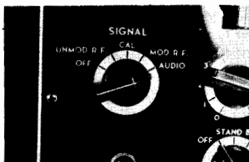
Fig. 8-11. Most signal generators have an audio-frequency output.
