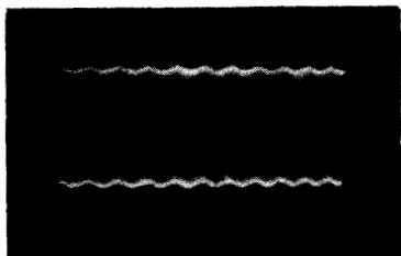
Fig. 8-2. Apparent AM limiter output, due to incidental FM.
