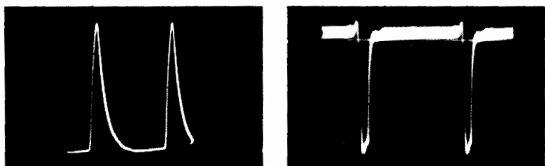
Fig. 4-15. Sync-separator outputs from two different receivers.
