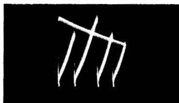
Fig. 9-8. Alternate peaks of the signal have different heights.
