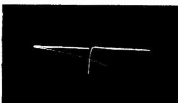
(B) Distorted (weakened) waveform when C is low in capacitance.
