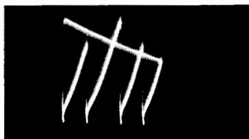
Fig. 4-11. Waveform with alternate symmetry.
