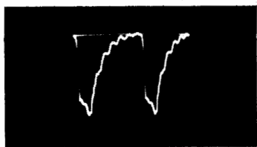
(B) Distorted waveform when C1 is leaky.
