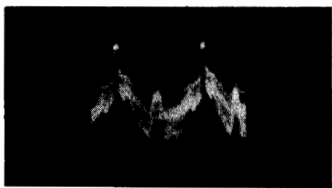
Fig. 3-2. Video waveform present at the looker point.
