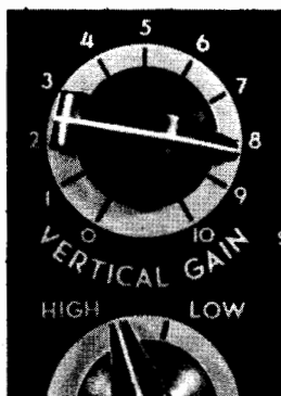
Fig. 1-15. Vertical-gain control incorrectly set.
