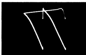
(A) Correct waveform, obtained with low-C probe.
